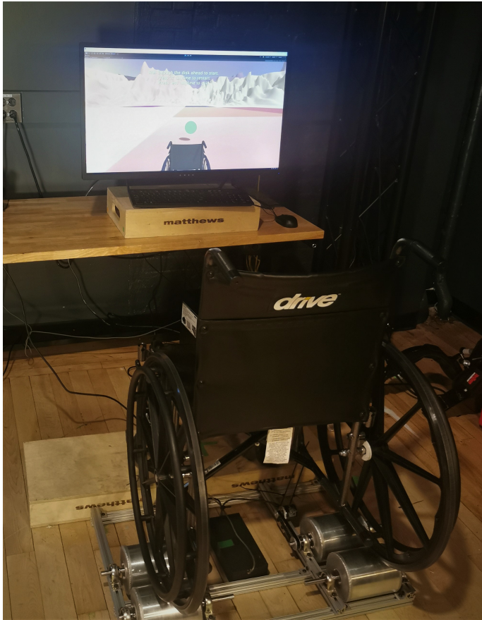
Fig. 7: The wheelchair is in front of a 2D screen and stands on the interface. The user’s wheel propulsion is translated into movement in the playground from Figure 3. The user is in the experience for eight minutes.
